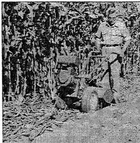
Photo 4-25: THIRD PASS – Go back over the stalks you knocked down from the opposite direction. This buries much of the residue 3"-to-4" deep.
